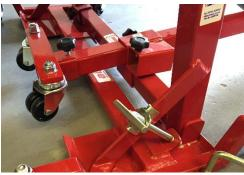
Slide the first arm a short way through the 3-way tube to allow the front wheel kit to be pushed over the end of the arm. Ensure the arm is fully inserted into the wheel kit and is touching the stopper bolt inside the wheel kit tube. Next tighten the thumb screw securley.
