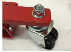
Fit both castors ensuring the bolts are inserted from the underside of the castor. Use 1x washer and 1x nyloc nut per wheel. Tighten securely with a spanner and the hex key provided. Note: Ensure all castors spin freely, if you find a castor not spinning freely, simple loosen the bolt slightly.
