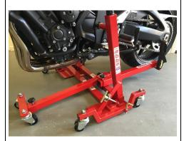
Operate the Front lift arm in the normal way (refer to instructions if unsure) by using the lifting strap so both wheels of the bike are elevated from the ground.
