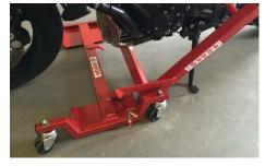
Before lifting, put your left foot in front of the Moto Glide to keep the Moto Glide in position. Operate the Superbike stand in the normal way pulling the lever forward. NOTE: You will be lifting the stand slightly higher than normal, so this will require a little extra effort to operate than when using the Superbike stand on its own.
