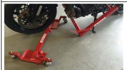
Once your Superbike stand is fitted in the normal way, slide the Moto Glide in between the front wheel and stand.
