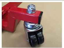
Fit all four castors to the Moto Glide, ensuring the bolt is inserted from the underside of the castor. Use 1x washer and 1x nyloc nut per wheel. Tighten securely with a spanner and the hex key provided. Note: Ensure all castors spin freely, if you find a castor not spinning freely, simple loosen the bolt slightly.
