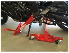
On certain motorcycles sliding the Moto Glide in between the stand and front wheel won't be possible. In this instance, slide the Moto Glide in behind the stand as shown above.
