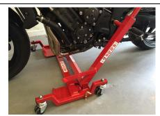
Stand the bike up vertical and raise the abba stand off the ground by pushing down on the handle when extended. Wheel the bike either forward or backwards (depending on locating position as mentioned previously). Locate the stand in the moto Glide with the side of the abba stand against the vertical stop on the Glide. Look over to the other side of the bike to ensure both sides are seated on the rear of the Moto Glide base
