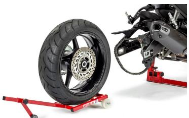
Once your wheel is free to be removed slide the wheel out of the bike while on the rizer.
