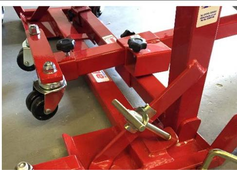
Slide the first arm a short way through the 3-way tube to allow the front wheel kit to be pushed over the end of the arm. Ensure the arm is fully inserted into the wheel kit and is touching the stopper bolt inside the wheel kit tube. Next tighten the thumb screw securely.
