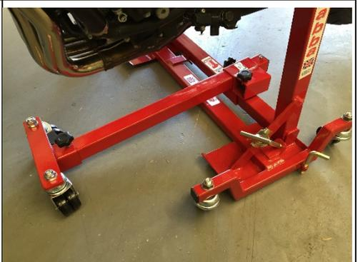
Slide the arm through **as far as possible** to ensure the wheel kit comes into contact with the ground.
