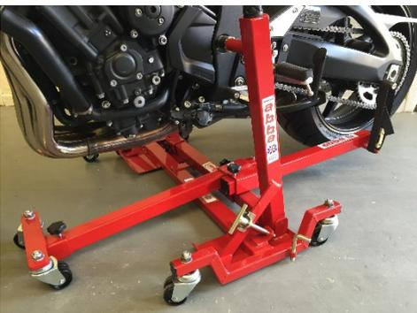
Operate the Front lift arm in the normal way (refer to instructions if unsure) by using the lifting strap so both wheels of the bike are elevated from the ground.
