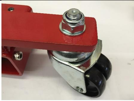
Fit both castors ensuring the bolts are inserted from the underside of the castor. Use 1x washer and 1x nyloc nut per wheel. Tighten securely with a spanner and the hex key provided. Note: Ensure all castors spin freely, if you find a castor not spinning freely, simply loosen the bolt slightly.
